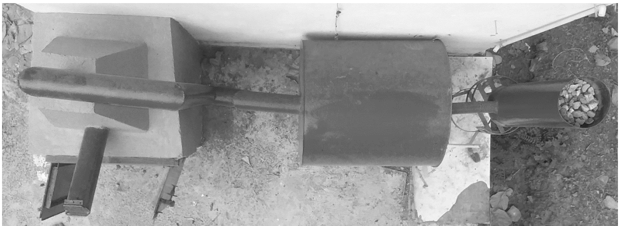
Plate 6 Liquid smoke production assembly (top view)
