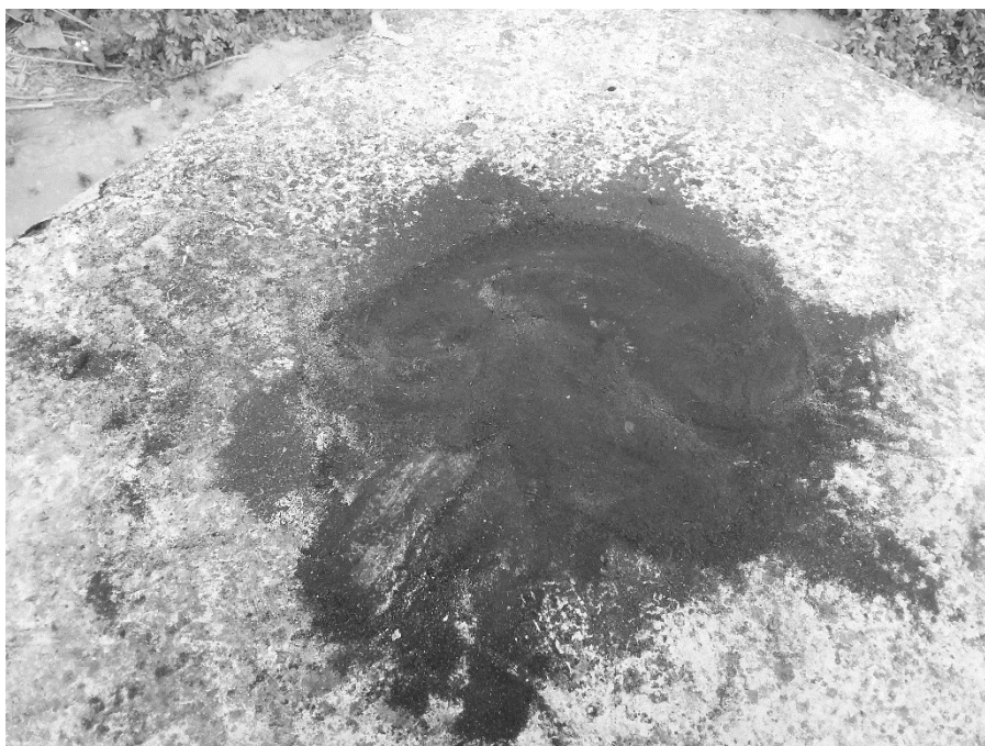
Plate 9 Sawdust after plate heating (pyrolysis)
