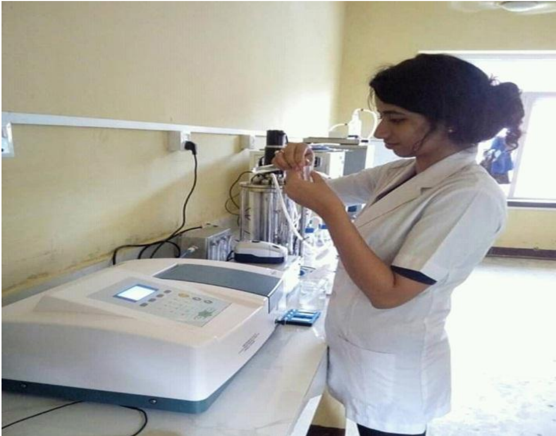
Plates 3: Study of free radical scavenging activity of flaxseed using spectrophotometer
