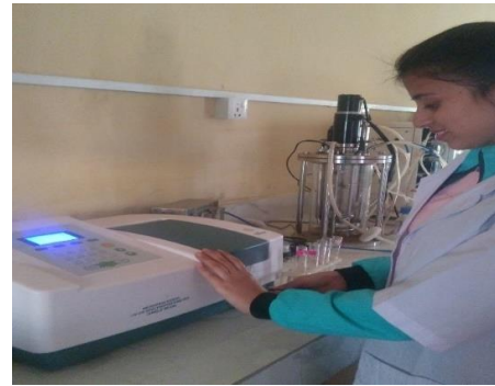
P4 Measuring absorbance of sel-roti sample
