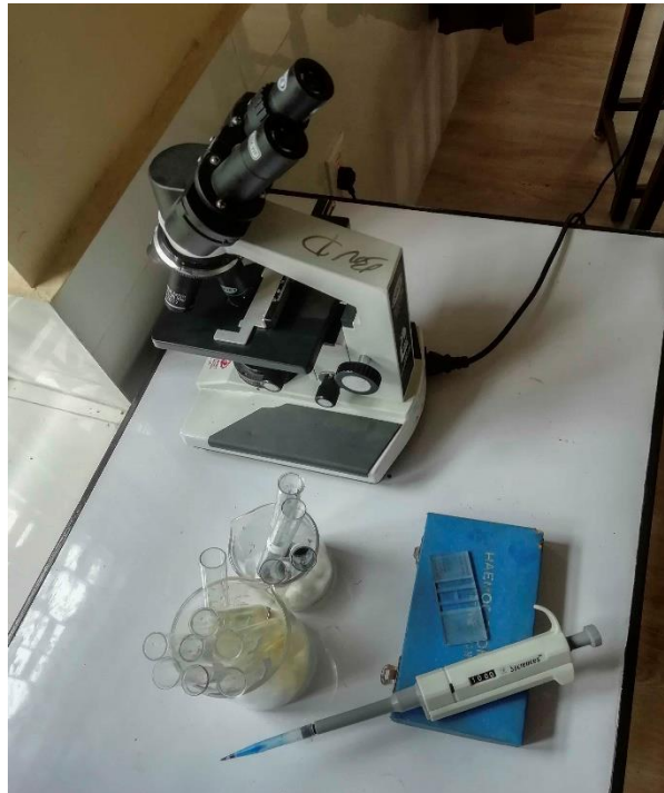
Setup for yeast cell count using hemocytometer
