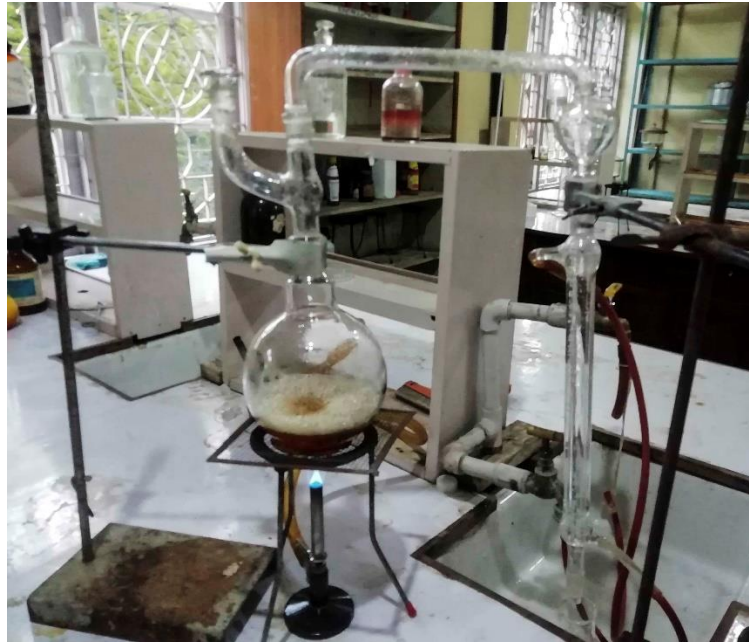
Distillation of metheglins to collect distillate for analysis
