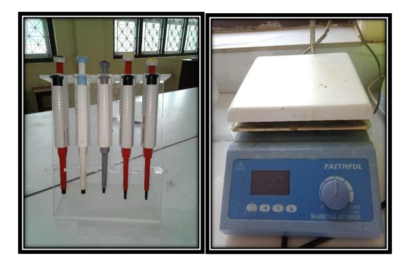
Plate 3: Micropipette and magnetic stirrer used during lab work
