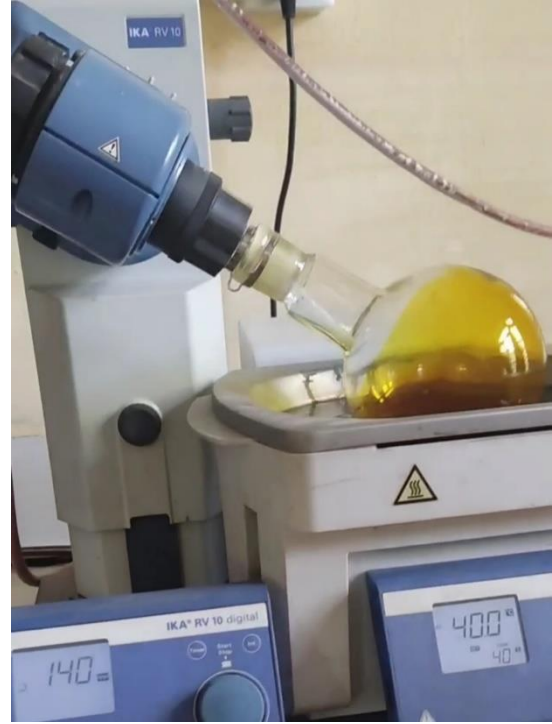
Plate 1 Ethanolic extraction process of spices using rotatory evaporator
