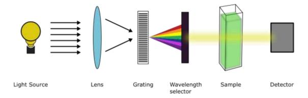
Figure 1: instrumentation of UV-Visible spectrophotometer
