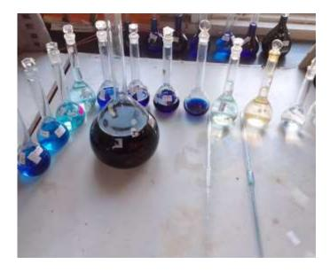
Photograph 4:Methylene blu solution of different concentration
