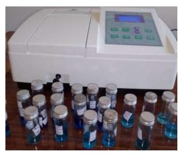
Photograph 5: UV-Vis Spectrophptometer
