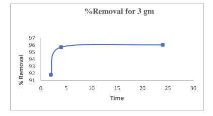
Figure 6: contact time vs removal% for 3gm sample:
