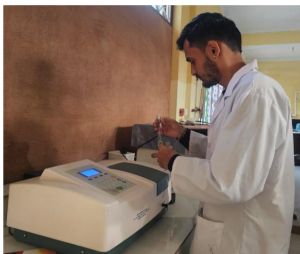
Fig. C.3 Spectrophotometric determination of TPC.
