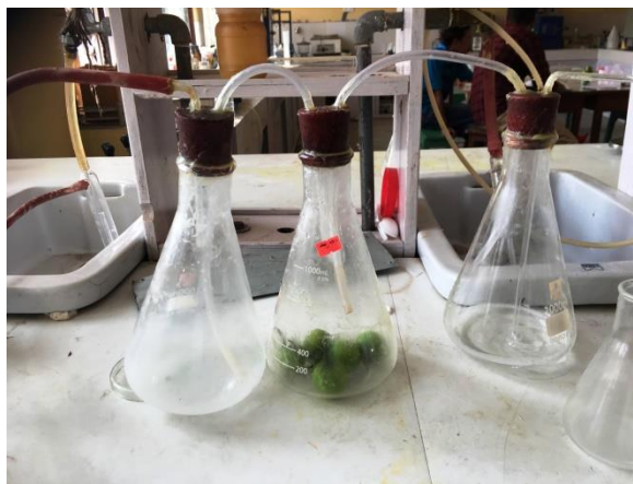
Plate. 3 Apparatus up for measuring Rate of respiration
