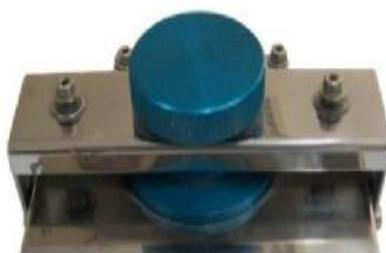
**Fig. 3.2** Sealing Cassette used in estimation of urinary iodine.
