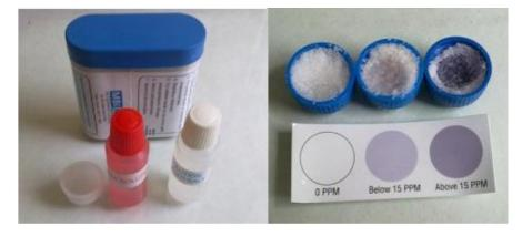
Fig. 3.3 Colour chart used to detect salt iodine concentration by rapid test kits.
