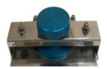
Fig. 3.2 Sealing Cassette used in estimation of urinary iodine.
