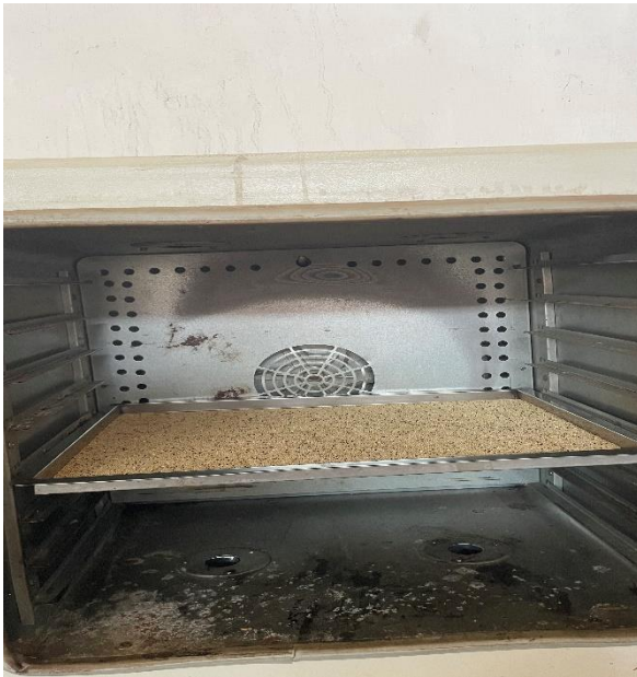
P1 Grain drying in cabinet dryer
