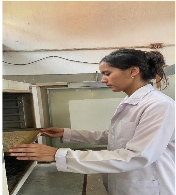
P1 Grain drying in cabinet dryer
