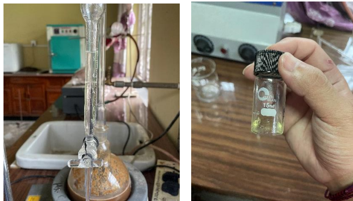
Plate 1 Extraction of essential oils using cleavenger apparatus
