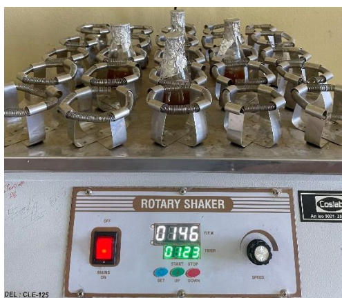
Plate 2 Mixing of the juice sample with essential oils using rotary shaker
