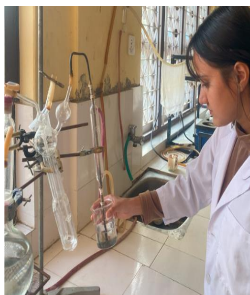
P4 Distillation in Kjeldahl's distillation set digestion for analysis of protein
