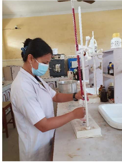
P2 Titration for oxalate determination
