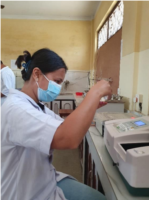
P1 Spectrophotometric determination of polyphenols
