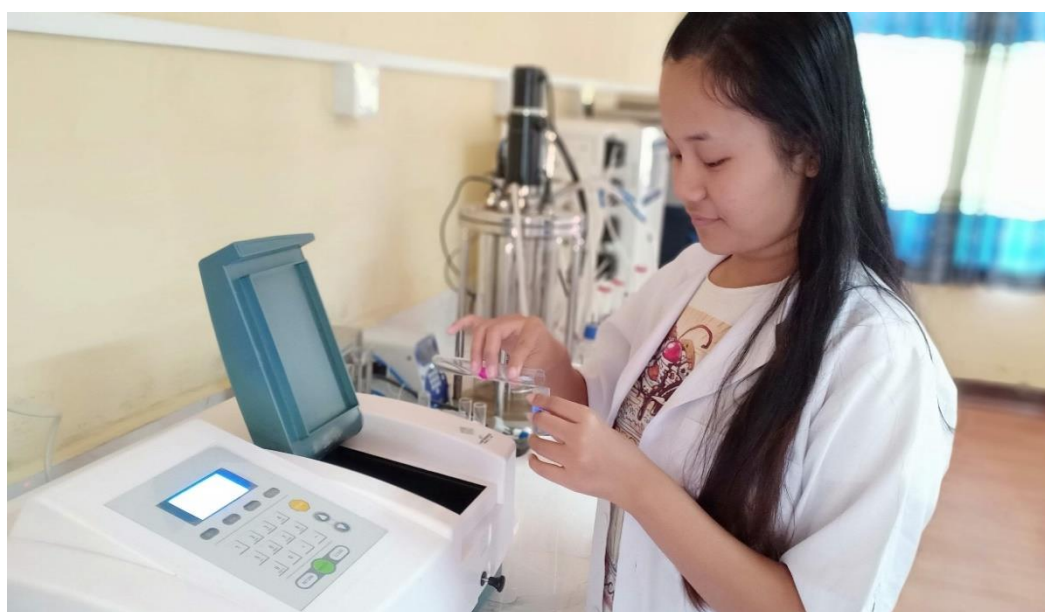
Plate 10: Study of free radical scavenging activity of fenugreek seed using spectrophotometer
