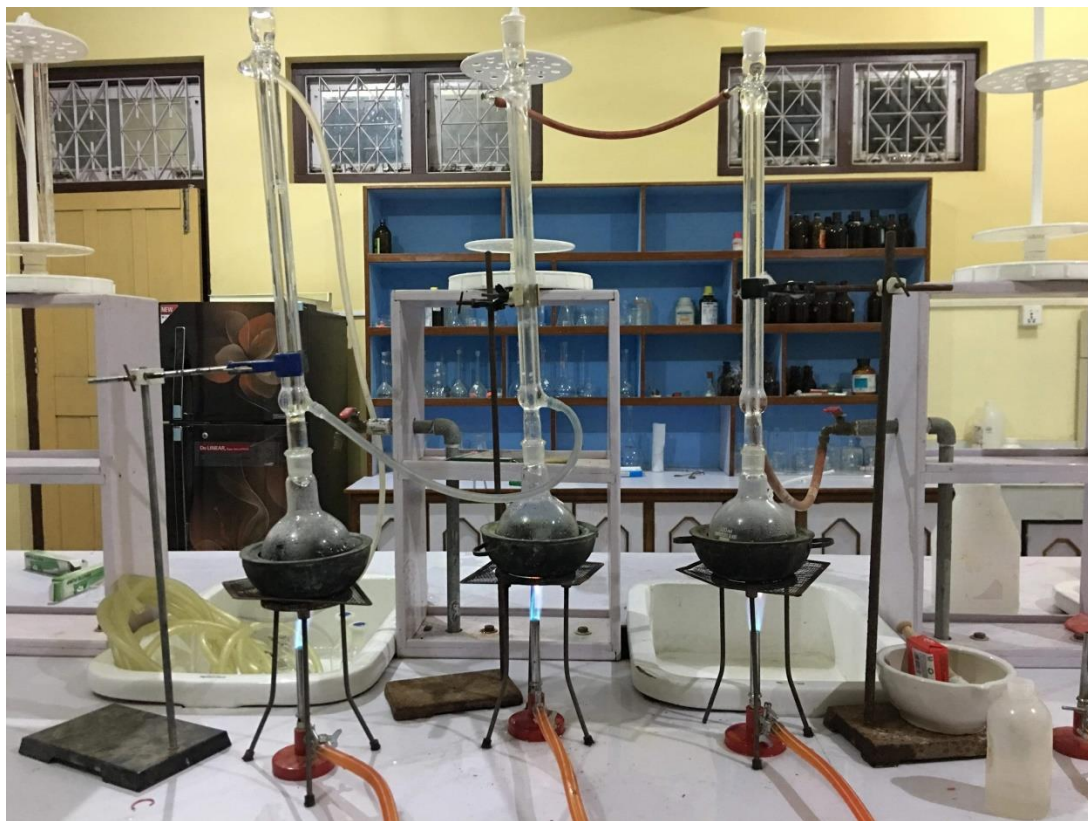
P 7. Performing acid hydrolysis connected with reflux condenser
