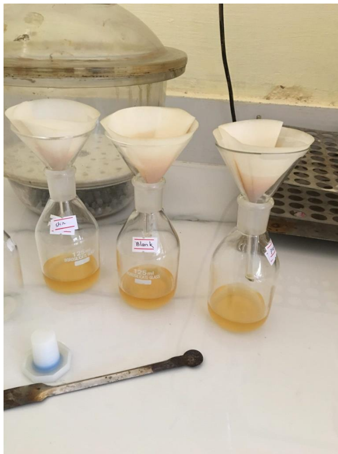
P 6. Performing the filtration of rice samples
