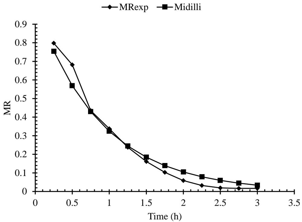
**Fig. 4.5** Experimental and predicted Moisture ratio variation with drying time of *gundruk* during cabinet drying at 50°C
