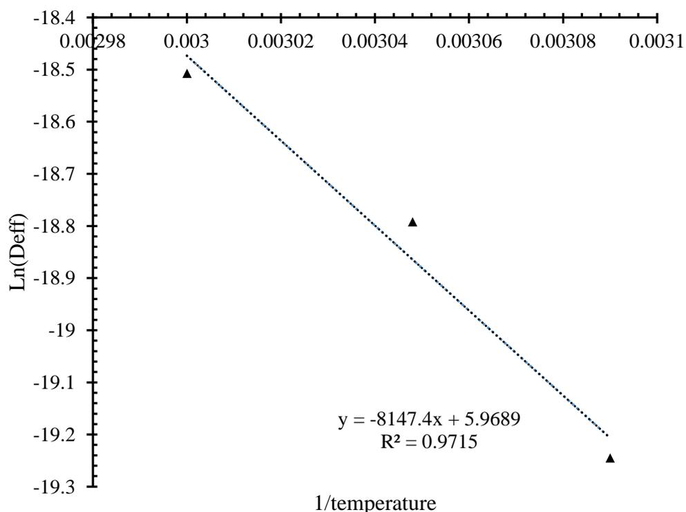
**Fig. 4.16** Arrhenius-type relationship between effective moisture diffusivity and the reciprocal of absolute temperature.
