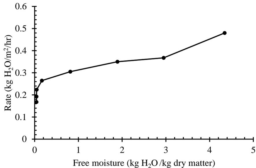
**Fig. 4.2** Drying rate curve of *gundruk* showing drying rate as a function of moisture content.
