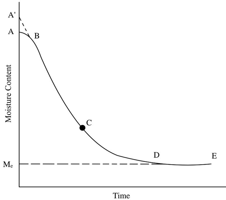
**Fig. 2.2** Drying curve showing moisture content as function of time
