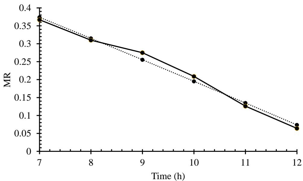
**Fig. 4.20** Experimental and predicted Moisture ratio variation with drying time for traditional solar dryer (Day 2)
