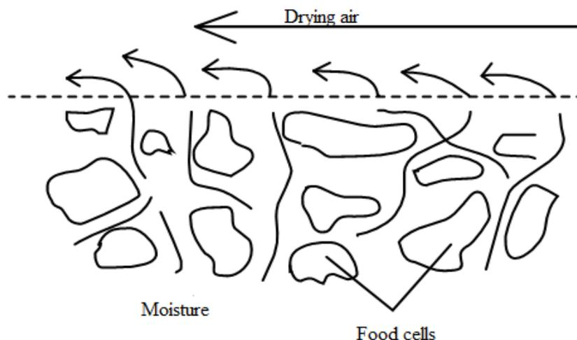
**Fig. 2.1** Movement of moisture during drying
