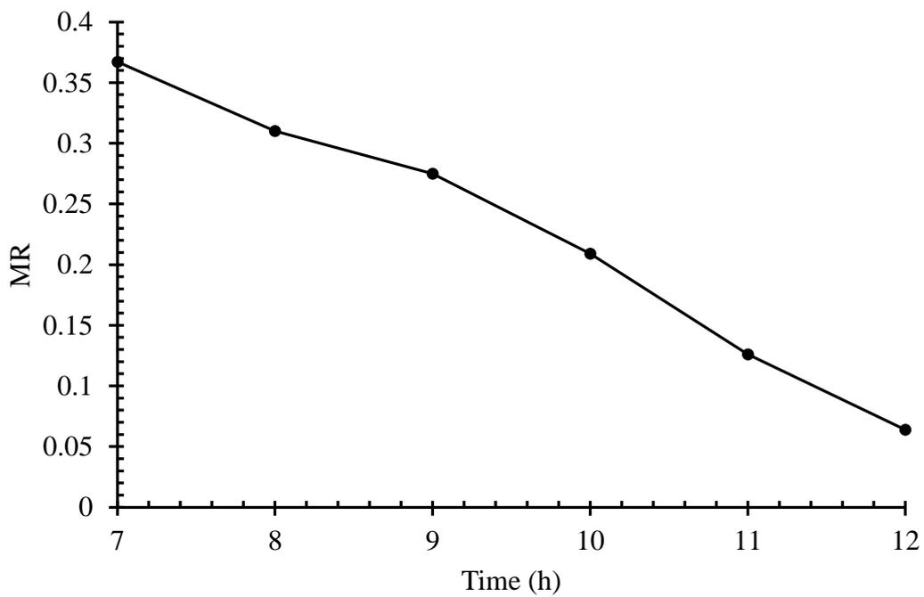
**Fig. 4.18** Variation of experimental MR with time during solar drying (Day 2)
