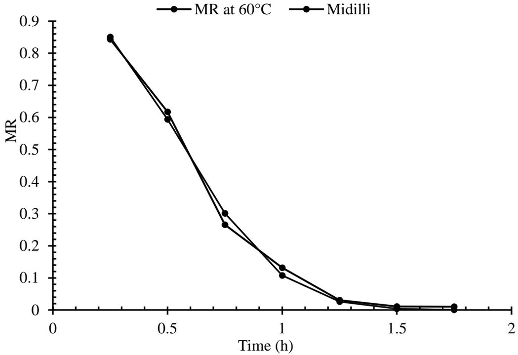
**Fig. 4.11** Experimental and predicted Moisture ratio variation with drying time of *gundruk* during cabinet drying at 60°C
