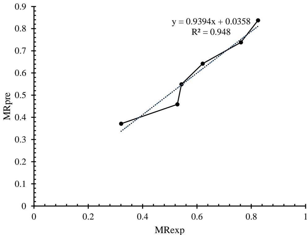
**Fig. 4.21** Theoretical vs Experimental Moisture ratio (Day 1)
