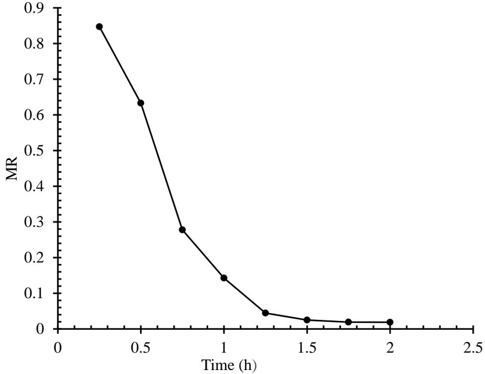
**Fig. 4.7** Variation of experimental MR with time at 55°C
