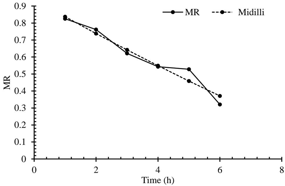
**Fig. 4.19** Experimental and predicted Moisture ratio variation with drying time for traditional solar dryer (Day 1)
