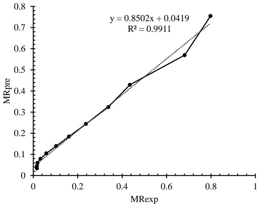
**Fig. 4.6** Predicted vs Experimental moisture ratio at 50°C.
