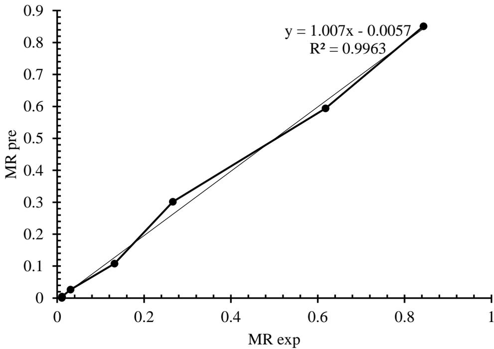
**Fig. 4.12** Predicted vs Experimental moisture ratio at 60°C
