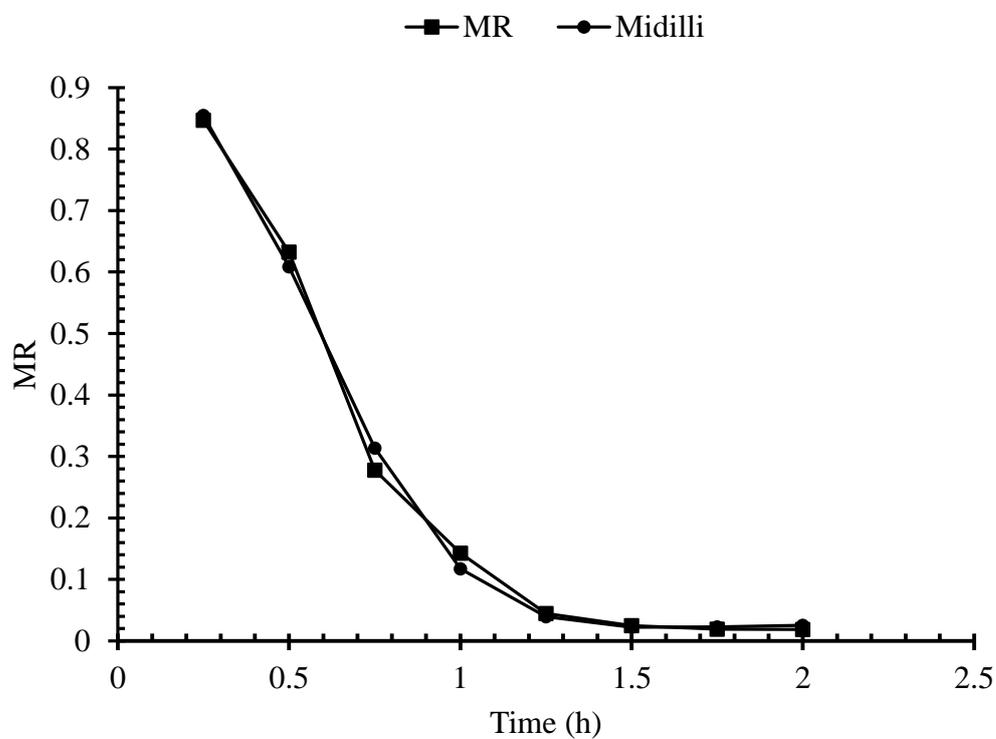
**Fig. 4.8** Experimental and predicted Moisture ratio variation with drying time of *gundruk* during cabinet drying at 55°C
