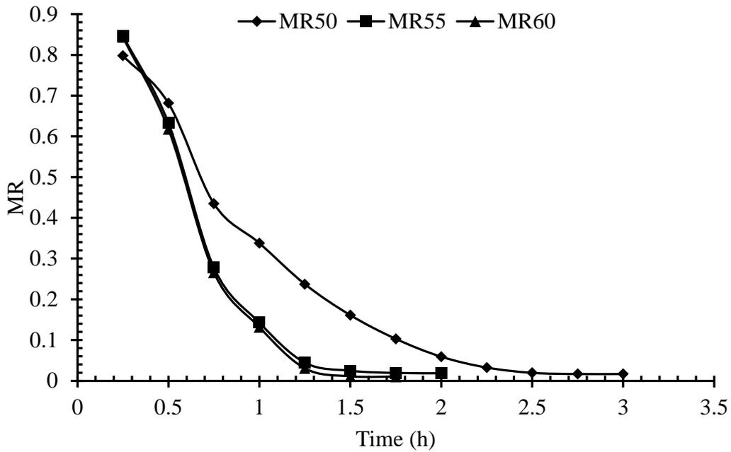
**Fig. 4.3** Variation of experimental MR at 50°C, 55°C, 60°C with time during cabinet drying.
