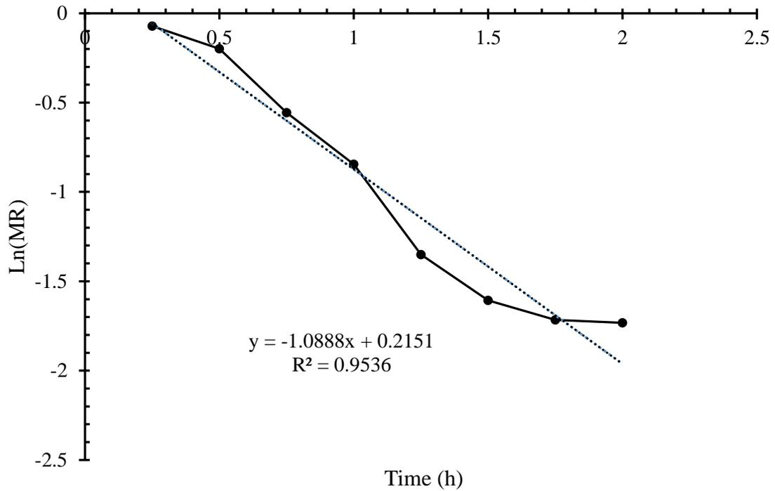
**Fig. 4.14** Graphical representation of Ln(MR) vs time at 55 °C
