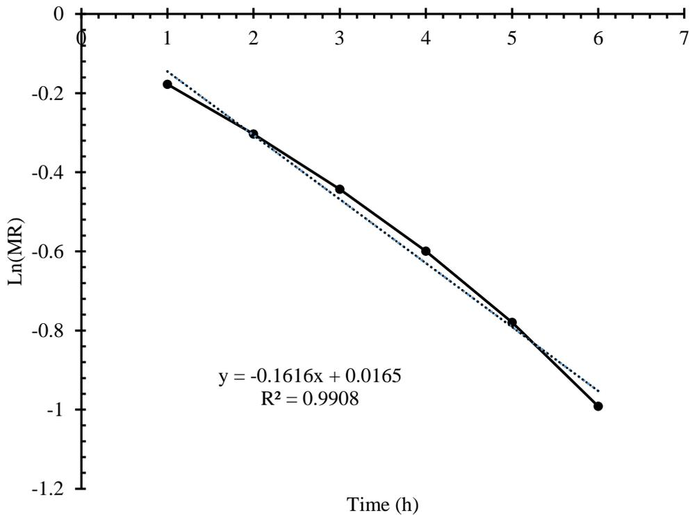
**Fig 4.23** Graphical representation of  $\ln(MR)$  vs. time during solar drying(day 1)
