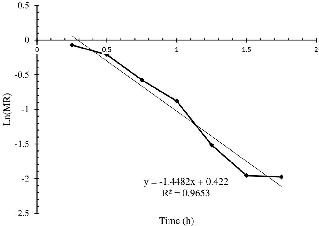
**Fig. 4.15** Graphical representation of Ln(MR) vs time at 60 °C
