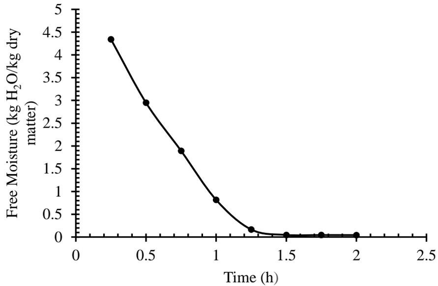
**Fig. 4.1** Drying rate curve of *gundruk* showing free moisture as a function of time
