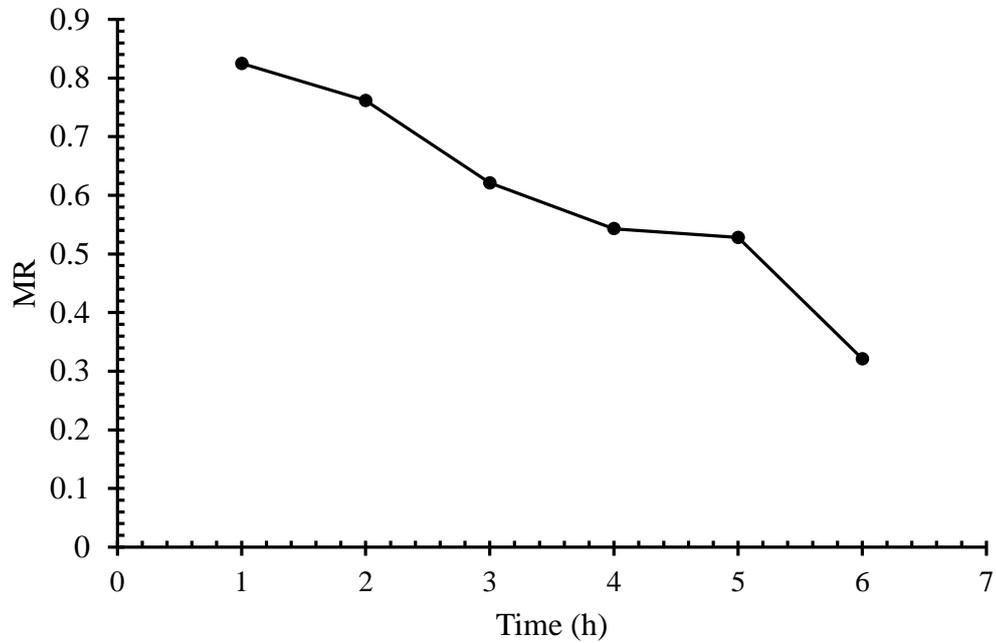
**Fig. 4.17** Variation of experimental MR with time during solar drying (Day 1)
