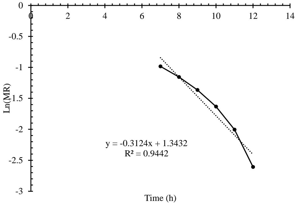
**Fig. 4.24** Graphical representation of Ln(MR) vs. time during solar drying (day 2)
