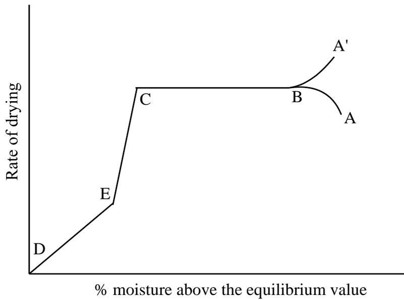
**Fig. 2.3** Drying Rate as a Function of Moisture Content
