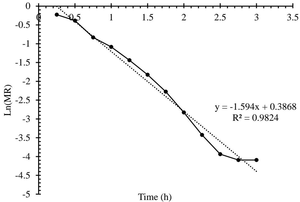
**Fig. 4.13** Graphical representation of Ln(MR) vs time at 50°C
