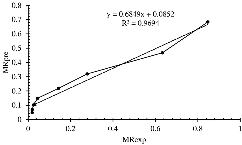
**Fig. 4.9** Theoretical vs. experimental moisture ratio at 55°C
