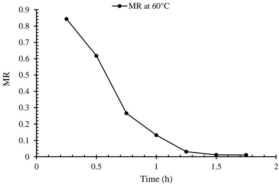
**Fig. 4.10** Variation of experimental MR with time at 60°C
