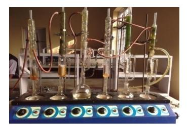
Plate 1: Fat extraction by Soxhlet apparatus
