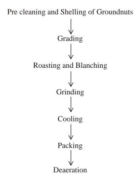
Fig. 2.5 Flow-chart for manufacturing process of peanut butter
