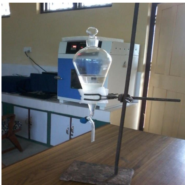
Photograph 5: Extraction of antimicrobial metabolites by using organic solvent (ethyl acetate) in a separating funnel
