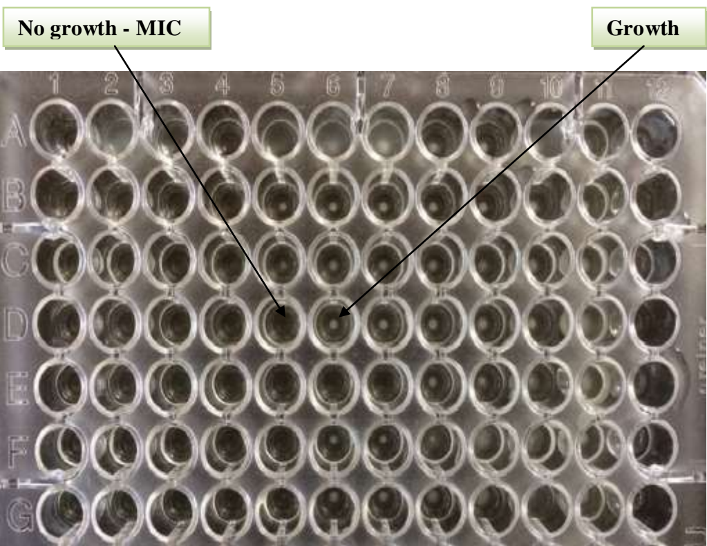
Photograph 6: MIC of vancomycin by Microbroth dilution method
