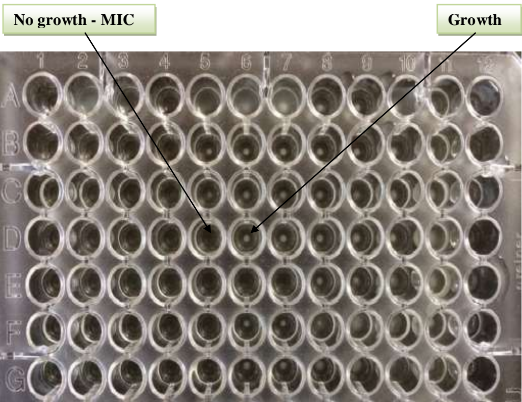
Photograph 6: MIC of vancomycin by Microbroth dilution method
