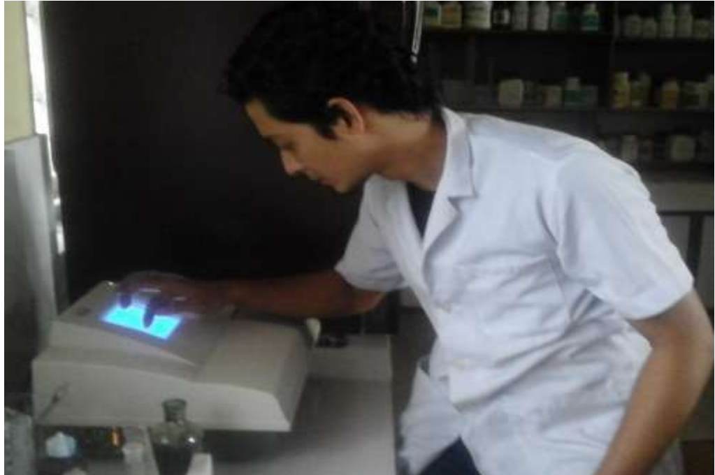
Photograph 4: Operating ELISA reader for determining biofilm OD
