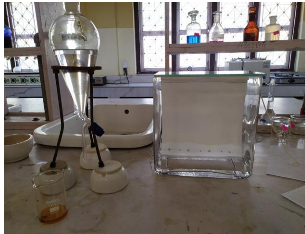
P3. Qualitative analysis of essential amino acids by paper chromatography
