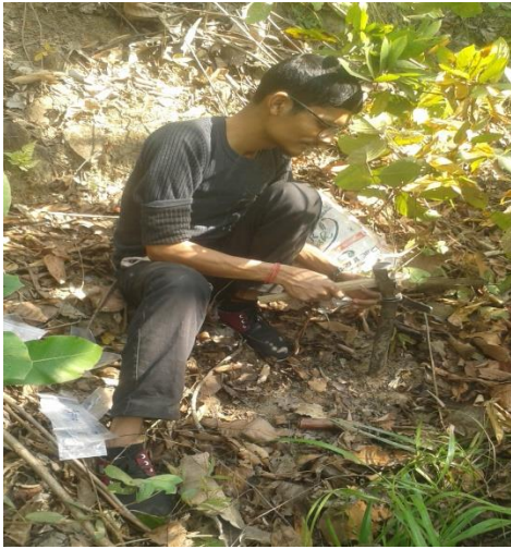
Fig: Drilling of Soil Corer to collect sample
