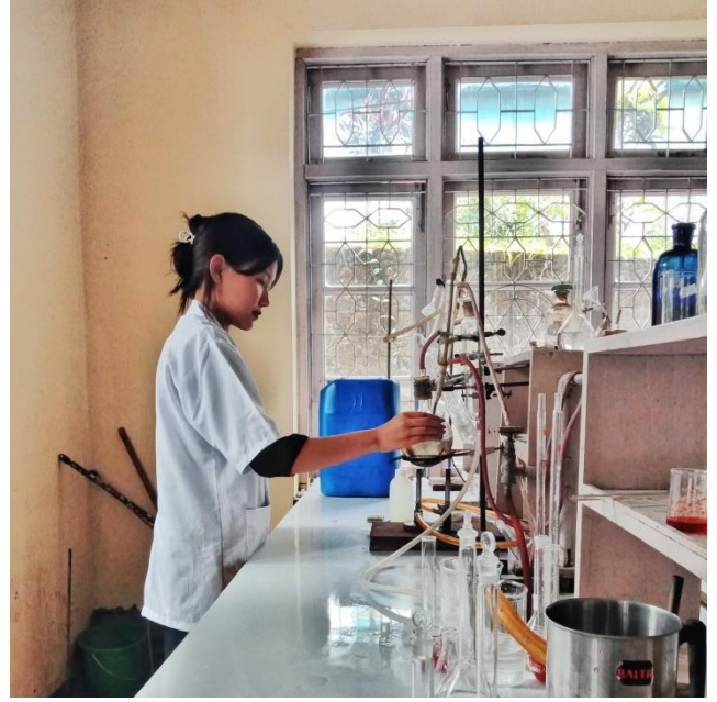
Plate 6. Distillation in Kjeldahl's distillation set
