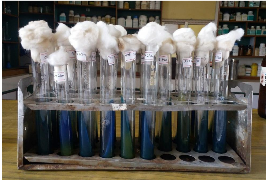
Photograph 3: Citrate Utilization Test (+ve for Klebsiella pneumoniae , -ve for Escherichia coli )
