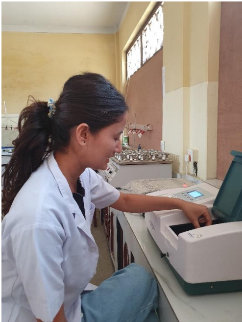
P1 Reading absorbance on spectrophotometer
