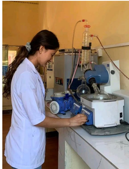
P2 Using rotary vacuum evaporator for extraction
