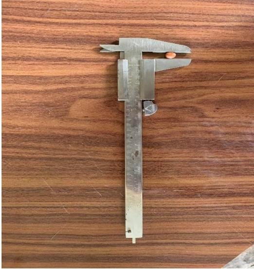
**Plate 1** Physical dimensions measurement
