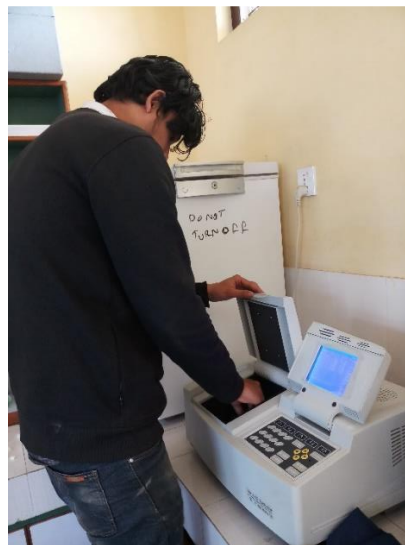
P2 Measuring absorbance in Spectrophotometer
